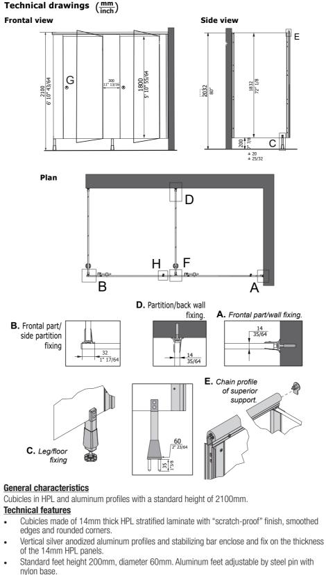
PDoors with self-approaching hinges with adjustable spacer, soft-close system, recessed • flush lock in AISI 316 stainless steel with indicator free/engaged and integrated emergency opening, vandal-proof solid round lever (inside).
